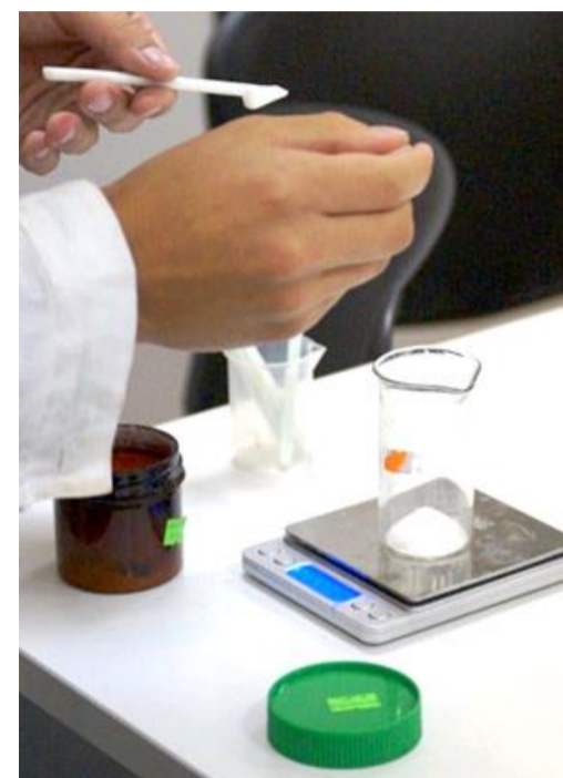
Fig. 5. Sampling preparation: weighting of cerium (III) sulfate (A) and potassium bromate (B).
