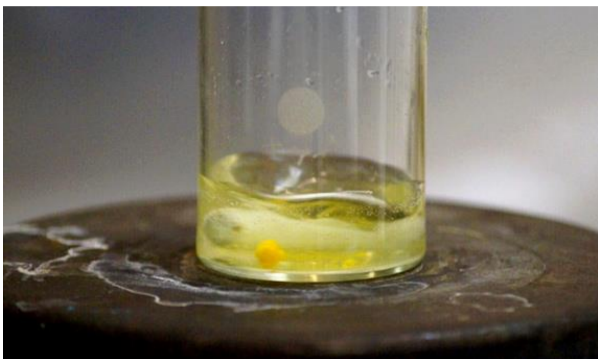
Fig. 6. Dissolution of reagents in sulfuric acid using of magnetic stirrer. Photo © S. Dolzhenko, A. Kadysheva
